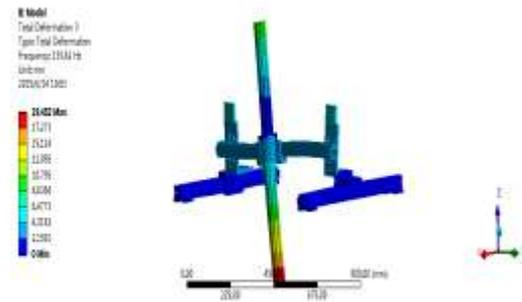
Figure 5. the third order mode of the mechanism
